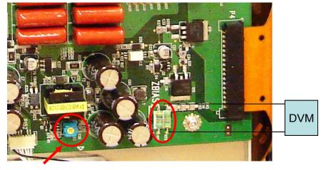
ZBIAS adjustment: On the Z-Sustain PCB With the DVM across R92 adjust the potentiometer till the DVM reads 93 vdc.
